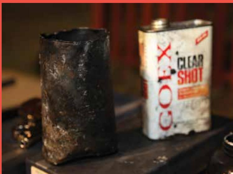
Cans of explosive powder used by murder suspect to start a fire. Can on left exploded during fire, can on right was thrown clear of fire.
