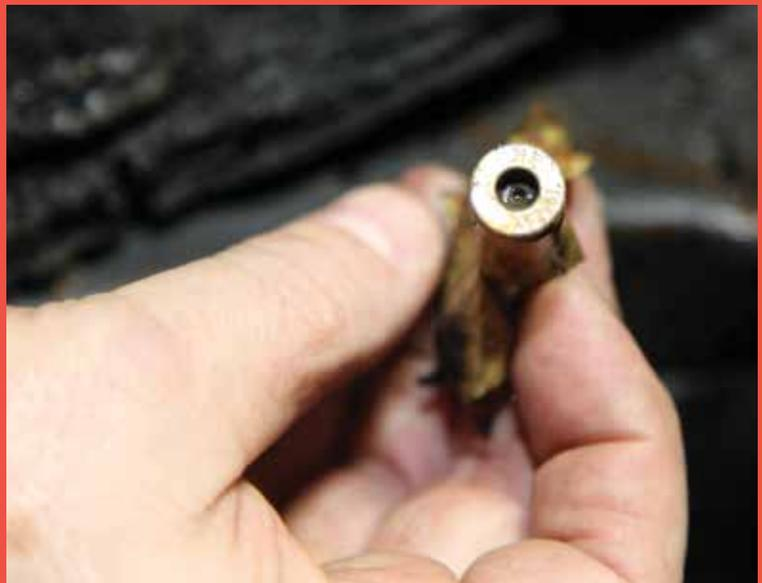
Primer expelled from live AK47 shell after exposure to fire (several thousand found in a single scene).
